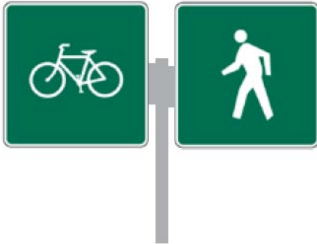
Figure 3-3. On side paths, mode specific guide signs for bicyclists (D11-1a) and pedestrians (D11-2) from Chapter 9 of the Wisconsin Manual on Uniform Traffic Control Devices manual may be used to identify paths for bicyclist and pedestrian use only. Credit: FHWA
