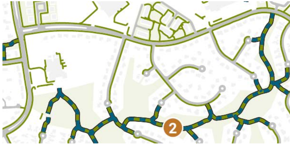
Figure 3-9. Bicycling and walking connections (2) that connect cul-de-sacs to busy roads and other destinations shorten travel distances for bicyclists and pedestrians. Credit: FHWA Achieving Multimodal Networks
