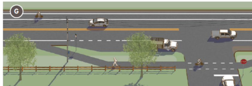
Figure 3-6. In this scenario, the shoulder is designated as a separated bike lane. Bicyclists are shifted laterally away from the roadway and separated from the travel or turn lanes by an unpaved buffer space.
